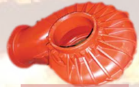
Wastewater pump housing 475 kg
